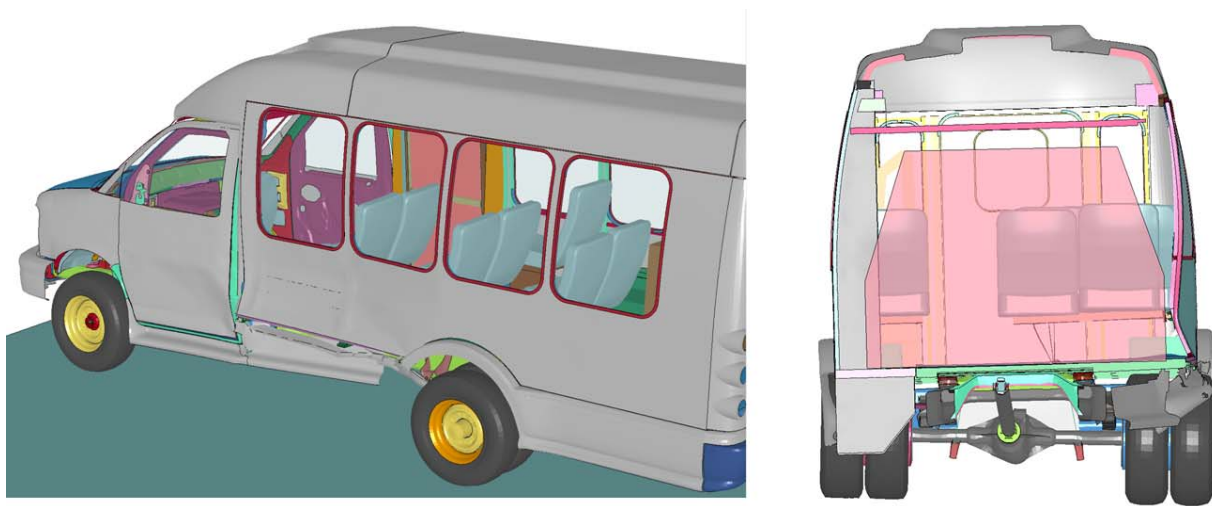
Figure 28: Final deformation of the bus body for the FE model with improved connections.
