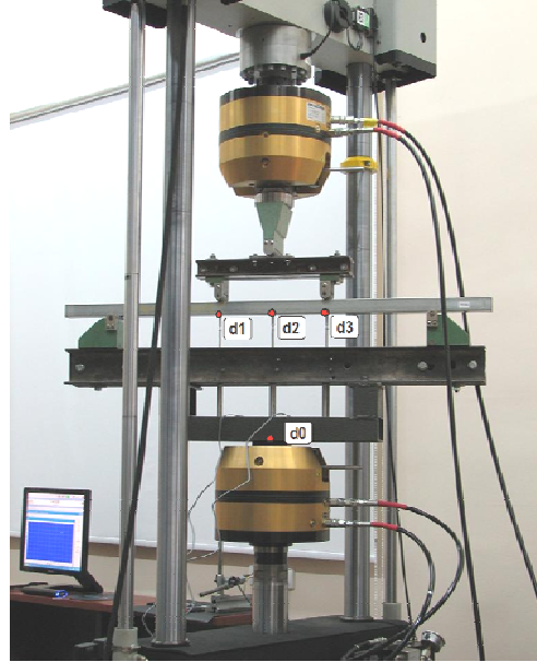
Figure 6: Testing apparatus for four point bending.
