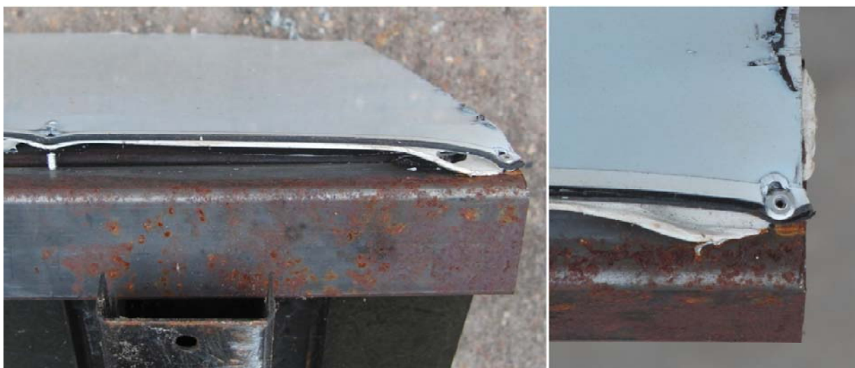
Figure 14: Localized damage to the skin as a result of testing.
