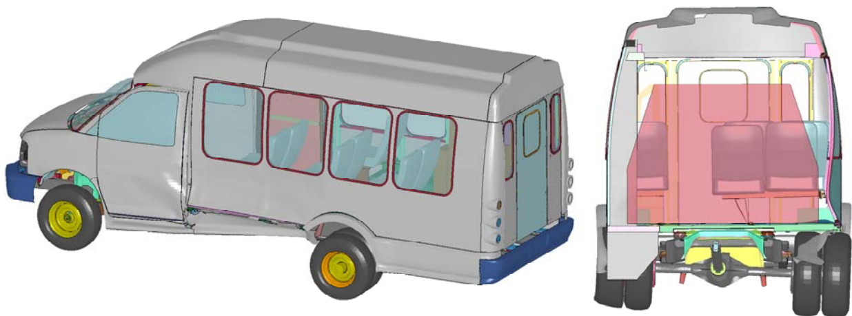
Figure 27: Final deformation of the bus body for the FE model without improved connections.
