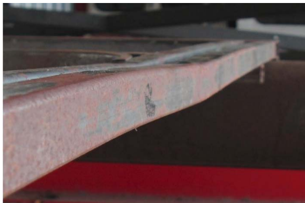
Figure 18: Close-up of slight local deformation in skinless wall sample.
