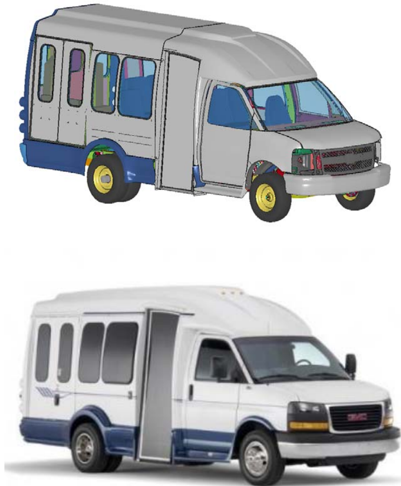
Figure 1: Finite element model (top) and an actual bus (bottom) of Turtle Top Terra Transport paratransit bus.
